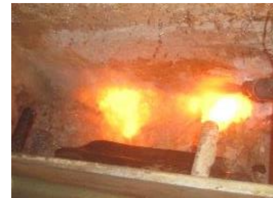
Critical area for glass leakage
