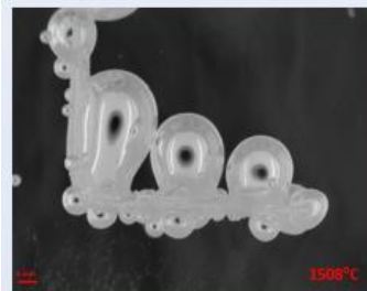
Fig. 5. The observation of the bubbles contraction during temperature drop, C/SO_4^{2-} = 9 . Bubbles in reduced amber glasses did not dissolve in the melt.
