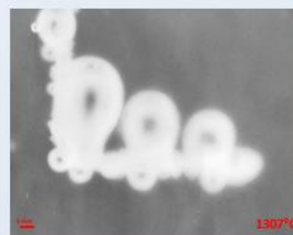
Fig. 5. The observation of the bubbles contraction during temperature drop, C/SO_4^{2-} = 9 . Bubbles in reduced amber glasses did not dissolve in the melt.
