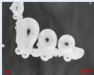
Fig. 5. The observation of the bubbles contraction during temperature drop, C/SO_4^{2-} = 9 . Bubbles in reduced amber glasses did not dissolve in the melt.
