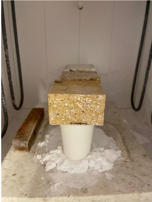
Alkaline penetration test set up
