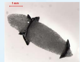
Silica Drip defect
