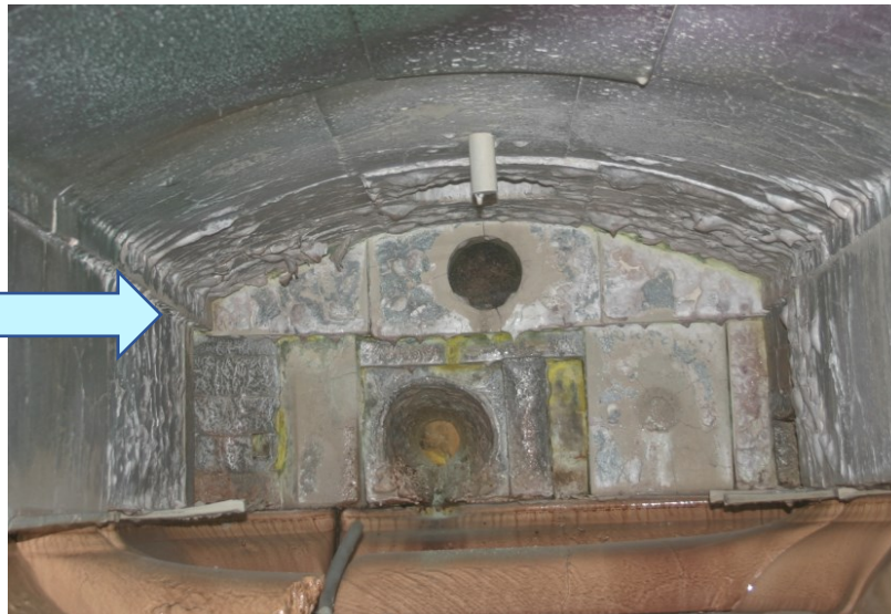
Oxy-fired soda-lime crown showing Fused Cast AZS exudate after ~4 years
